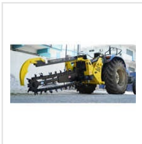
Rudra 100 Single Chain Compact Trenching
