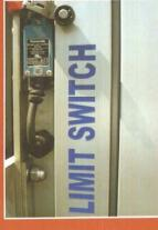
A high quality limit switch ensures cut off the power supply when platform reaches its optimum height. Safe control voltage (24 V) is in the circuit
