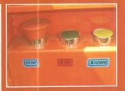
A pendent with all controls and emergency stop is provided on the platform which ensures independent working by the operator and after pushing the lock push button, no one can operate the platform from the floor, which ensures 100% safety while working on heights.
