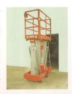
The platform is light weight and very easy to move any where by a single person only. Here it shows the open position of rallings on platform which needs much height of doors to enter.
