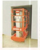
Railings can be folded in the platform, so, it can enter in low height gates, even around 2mtr. clear space, which makes this machine very handy & can have access any where in plants, godowns etc., conveniently.
