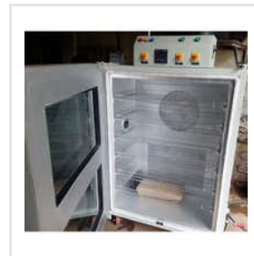
MS PCB Curing Oven
