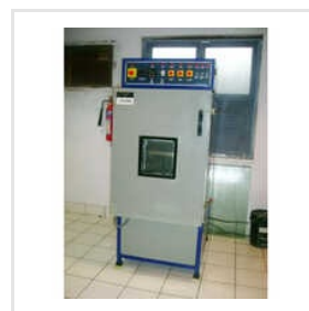
440 VAC Humidity Chambers
