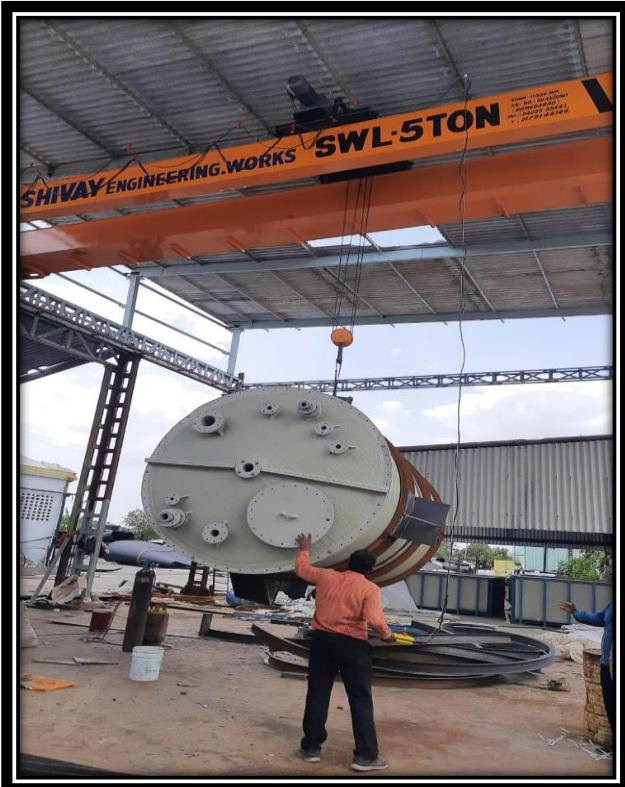
**DOUBLE GIRDER CRANES** are used for heavier loads and longer span. They offer the advantages of low headroom as the hook can be lifted up between the girders. All components are selected for 'crane duty applications'. Double Girder Cranes form a major amount of our annual orders. Depending on the span of the factory shed, the Double Girder Crane can be manufactured either with a Single Drive or a Twin Drive system.
