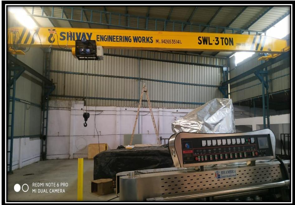
We manufacture **Single Girder Cranes** in different configurations : I-Beam type and girder/box type. Each configuration can be provided with twin/central drive. Decision regarding the configuration is made depending upon the shed dimensions and lifting requirements of the client. Electric Wire Rope Hoist are used on these cranes.
