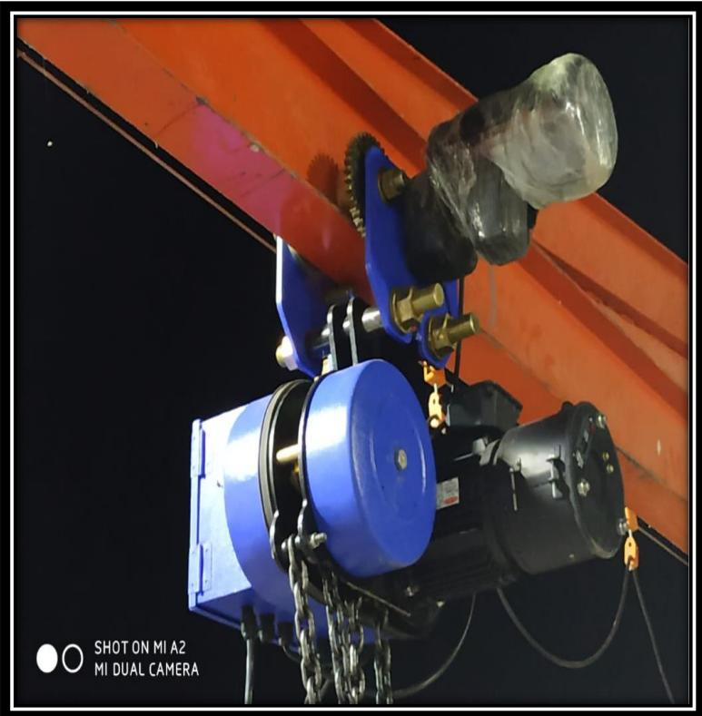
**0.5 Ton To 10 Ton** Chain hoists are compact, robust & elegant in appearance. We can manufacture Chain Hoists to suit your application requirements. Chain Electric Hoist are designed in accordance with IS-3938. Hoists are designed in modular giving positive Splash Lubrication. Motors are squirrel cage induction confirming to IS-325.
