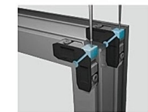
销钉注胶工艺 Pin glue injection process
