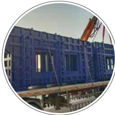
Box Culvert Mould
