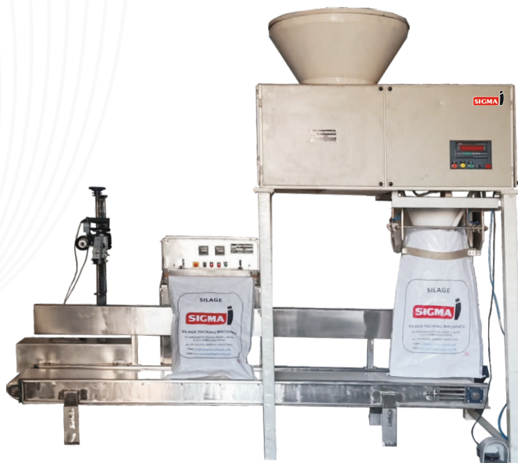
Powder Bag Filling with Stitching conveyor
