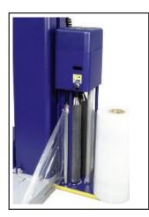
Fixed-rate powered pre-stretch carriage (150-200-250%), with manual wrapping tension adjustment possibilities using the potentiometer. Film tensioning is electronically controlled by a load cell and amplifier that control the film unwinding motor inverter. An electromagnetic clutch puts the rubber coated pre-stretch rollers in idle gear to allow for fast and simple film clamp at the beginning of each
