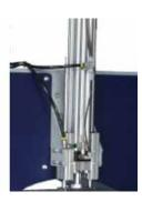
The vertical pressure units automatically settle in order to ensure correct stabilisation of the product during strapping. The length of the run can be adjusted manually to ease positioning of the pressure units on the products of different heights.
