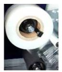
The Spool carriage unit has a direct breaking transmission roller and is adjustable at any time it also eases spool loading and film insertion to a maximum. The spool carriage device is equipped with locking and quick release of the spool.
