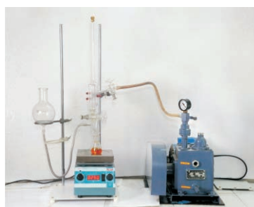
Extraction Method 7.3 of IEC 60567
