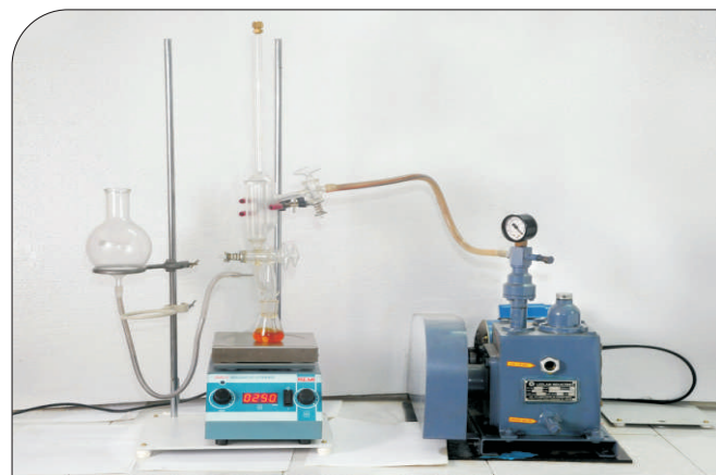
Extraction Method 7.3 of IEC 60567
