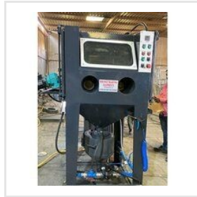
PB 9182 Pressure Blast Machine
