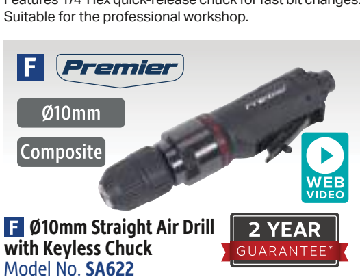
F 10mm Straight Air Drill with Keyless Chuck Model No. SA622 Composite cover moulded around lightweight aluminium alloy housing reduces effects of chill on operator's hands and provides added control. Air motor with quality bearings for smooth and powerful operation. Exhaust outlet adjusts 360°, keeping airflow away from operator. Safety trigger prevents inadvertent operation. Fitted with 10mm Jacobs keyless chuck for fast bit changes. Suitable for the professional workshop.
