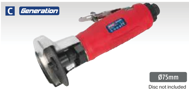
C Ø75mm Air Cut-Off Tool Model No. GSA25 Generation Series air cut-off tool. Contoured handle insulates user from chill and vibration. Metal disc guard and rear air exhaust can be rotated 360°, giving operator added protection. Includes throttle safety device. Cutting disc not included.
