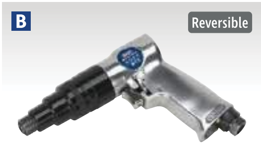
B Pistol Reversible Grip Air Screwdriver Model No. SA58 Pistol grip style, air operated screwdriver with reverse control. Positive clutch gives up to 115lb.in of torque. Suitable for assembly/dismantling and general production work. Features 1/4"Hex quick release chuck for fast bit changes.
