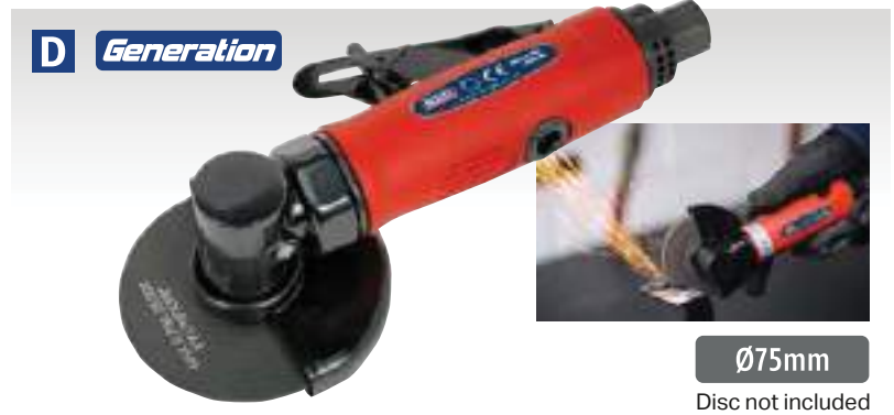
D Ø75mm Air Cut-Off Tool - Straight Model No. GSA26 Generation series air cut-off tool. Contoured handle insulates user from chill and vibration. Unlike conventional cut-off tools, the cutting disc is in-line with the handle for easier directional control. Metal disc guard and rear air exhaust can be rotated 360° giving operator added protection. Includes 4-position air valve and safety release trigger control to prevent accidental operation. Cutting disc not included.
