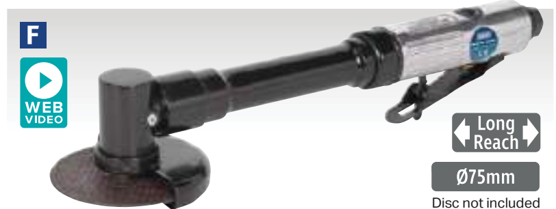
F Ø75mm Long Reach Air Cut-Off Tool - Straight Model No. SA2501 Extended reach cut-off tool is especially suitable for cutting off rear axle and exhaust tubes/brackets. Additionally suited to cutting off side frames or door sills. Fitted with metal safety guard and throttle safety device to prevent accidental operation. Cutting disc not included.
