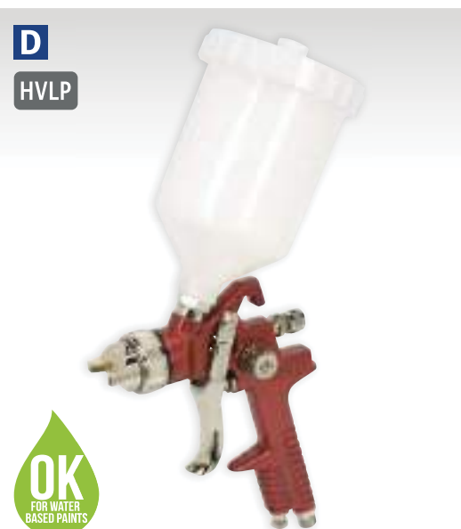
D Workshop Series HVLP Gravity Feed Spray Gun 1.3mm Set-Up Model No. HVL741 Suitable for applying top coats. Round/flat fan control allows spray pattern to be adjusted for any job. Brass air cap with stainless steel needle and nozzle make this HVLP gun suitable for water based paint. Standard Set-Up: 1.3mm Available Set-Ups: 1.2, 1.4, 1.7, 2mm Recommended Air Pressure: 43psi Air Consumption: 15cfm Pot Capacity: 600ml
