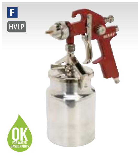
F Workshop Series HVLP Suction Feed Spray Gun 1.7mm Set-Up Model No. HVL740 Round/flat fan control allows spray pattern to be adjusted for any job. 1.7mm Set-up is ideal for applying primers, undercoats and adhesives. Brass air cap with stainless steel needle and nozzle make this HVLP gun suitable for water based paint. Standard Set-Up: 1.7mm Available Set-Ups: 1.2, 1.3, 1.4, 2mm Recommended Air Pressure: 43psi Air Consumption: 16cfm Pot Capacity: 800ml
