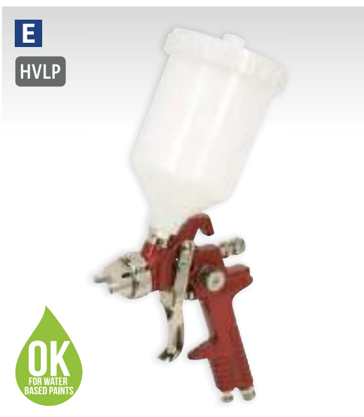
E Workshop Series HVLP Gravity Feed Spray Gun 2mm Set-Up Model No. HVL742 Ideal for applying high viscosity paints such as primer or undercoat. Round/flat fan control allows spray pattern to be adjusted for any job. Aluminium air cap with stainless steel needle and nozzle make this HVLP gun suitable for water based paint. Standard Set-Up: 2mm Available Set-Ups: 1.4, 1.7mm Recommended Air Pressure: 43psi Air Consumption: 15cfm Pot Capacity: 600ml
