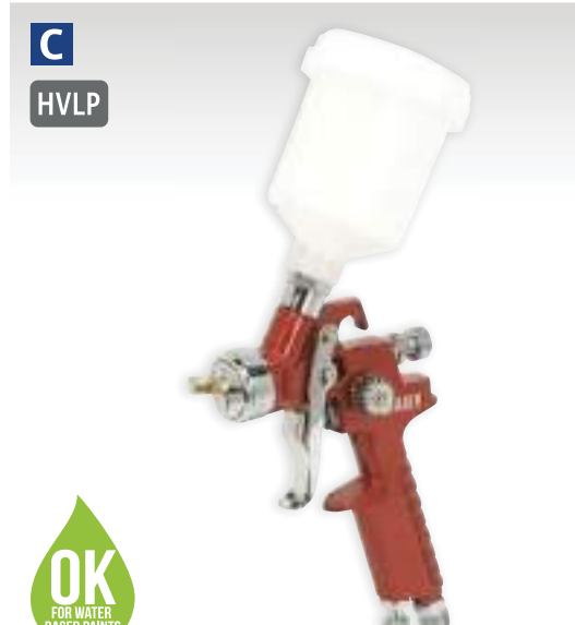
C Workshop Series HVLP Gravity Feed Touch-Up Spray Gun 0.8mm Set-Up Model No. HVL731 Ideal for blowing-in small areas of panel where fine control of paint and air is necessary. Brass air cap with stainless steel needle and nozzle make this HVLP gun suitable for water based paint. Standard Set-Up: 0.8mm Available Set-Up: 1mm Air Pressure: 43psi Air Consumption: 9cfm Pot Capacity: 100ml
