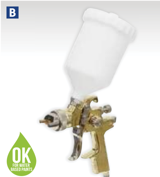
B Gold Series Gravity Feed Spray Gun 1.4mm Set-Up Model No. S701G Suitable for applying finishing coats. 2-Stage trigger control and 600ml plastic gravity feed pot. Adjustable spray width and fluid flow. Maintenance tools supplied. Suitable for use with water based paints. Alternative set-ups available separately. Standard Set-Up: 1.4mm Available Set-Ups: 1.7, 2mm Recommended Air Pressure: 43psi Air Consumption: 16cfm Pot Capacity: 600ml
