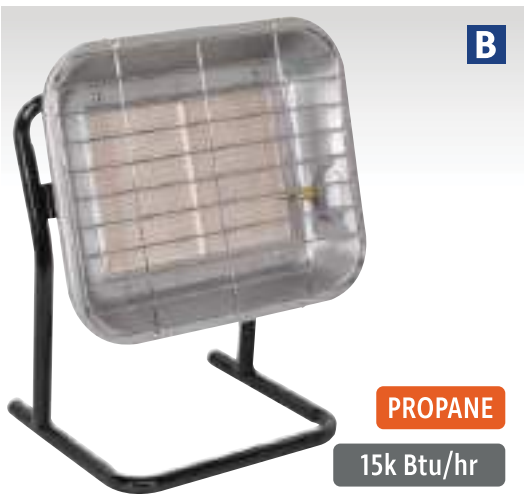
B 15,354Btu/hr Space Warmer® Propane Heater with Stand Model No. LP14 Ceramic plaque type heater. Steel tube stand with built-in handle. Adjustable output from 10,250 to 15,354Btu/hr. Supplied with 37mbar fixed regulator and 1.5m gas hose. Fuel: Propane Output: 10,250-15,354Btu/hr Fuel Consumption: 0.22-0.33kg/hr
