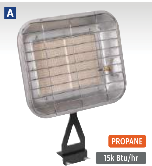
A 15,354Btu/hr Space Warmer® Propane Heater - Bottle Mounting Model No. LP13 Ceramic plaque type heater. Mounts on the rim of a propane cylinder. Adjustable output from 10,250 to 15,354Btu/hr. Supplied with 37mbar fixed regulator and 700mm gas hose. Fuel: Propane Output: 10,250-15,354Btu/hr Fuel Consumption: 0.22-0.33kg/hr
