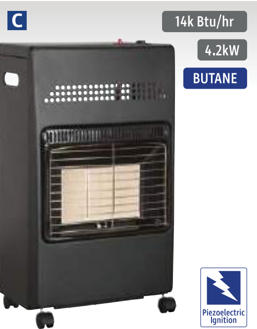
C 4.2kW Cabinet Gas Heater Model No. CH4200 Ceramic plaque cabinet heater ideal for office or home use. Accepts 15kg Butane bottle (not included) which fits into the rear of the unit. Features piezoelectric ignition, removing the need for batteries. Three heat output settings ranging from 1.55 to 4.2kW (5,288 to 14,330Btu/hr). Safety features fitted include a flame failure device, anti-tilt switch and oxygen depletion system. Supplied with hose and regulator. Fuel: Butane Output: 1.55/2.9/4.2kW(5,288-14,330Btu/hr) Fuel Consumption: 0.11/0.2/0.305kg/hr Overall Size (W x D x H): 430 x 295 x 750mm
