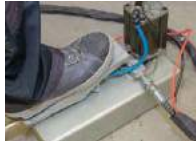
Foot operated lifting & lowering.
