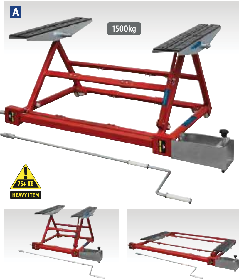
A 1500kg Portable Pivot Car Lift Model No. PPL01
