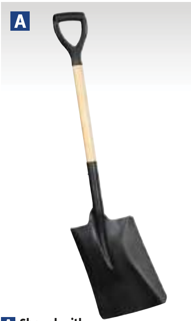
A Shovel with 710mm Wooden Handle Model No. SH710 Tough, pressed carbon steel shovel head tempered for extra strength. Fitted with hardwood ash handle. Manufactured to BS 3388. Length: 1020mm Handle: 710mm Blade: 260 x 340mm
