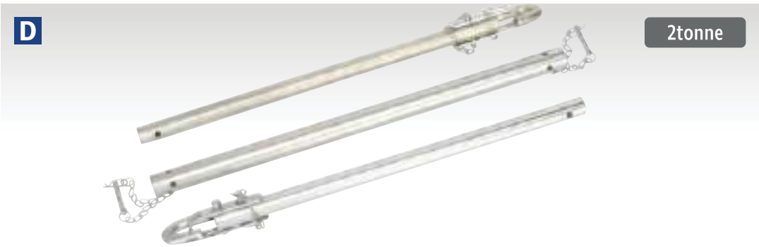
D Tow Pole 2000kg Rolling Load Capacity Model No. TPK252 2tonne Rolling load capacity tow pole. Steel sections clip together and fix with spring clips. Hooks feature sliding locking mechanism to prevent disengagement during towing/overrun. Maximum Rolling Load Capacity: 2tonne Length: 2m
