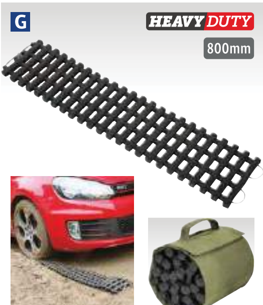
G 800mm Vehicle Traction Track Model No. VTR02 Heavy-duty vehicle traction track designed to prevent wheels spinning on snow, sand and mud. Flexible PVC design allows track to sit smooth against uneven surfaces. Fitted with galvanized steel cable and deep ribbed slatted cleats providing maximum grip. Each track can support a maximum safe working load of 3.5tonne. Supplied as singles in canvas storage pouch. Length: 800mm Width: 220mm Safe Working Load: 3.5tonne
