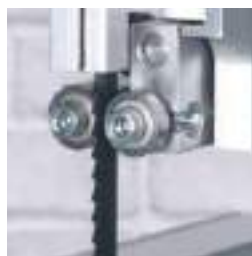
Ball-bearing blade guides for smooth operation*.
