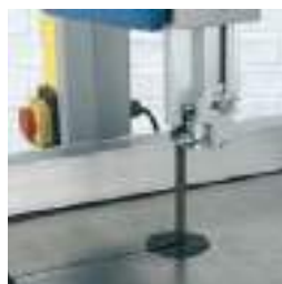
Adjustable height blade guide assembly.
