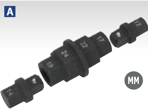
A 3pc Motorcycle Spindle Tool Set Model No. MS008 Prevents spindle from spinning when tightening or loosening wheel nut. Use appropriate socket on free end of tool to hold spindle. Six sizes to fit a variety of motorcycle makes and models. Spindle Sizes: 12, 14, 17, 19, 22, 24mm
