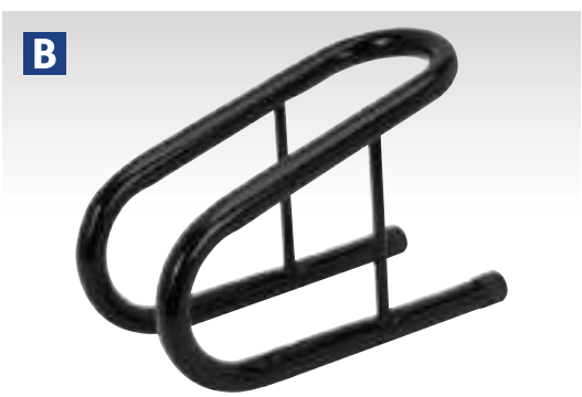
B Motorcycle Wheel Chocks Model No. SEE BELOW Black powder coated heavy-duty tubular frame. Pre-drilled holes allow chock to be bolted to either floor or trailer to prevent movement while being worked on or transported. Model No: Maximum Tyre Width: WC06 95mm WC07 140mm WC08 165mm
