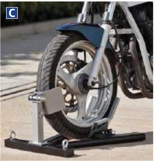
C Heavy-Duty Motorcycle Front Wheel Chock Model No. FPS7 Tubular wheel chock supports the front wheel of the motorcycle when in transit or storage. Fully adjustable to fit wheels 15"-21"(380-535mm). Features a pivot clamp which locks the front wheel securely by the motorcycle weight. Chock can be used freestanding or fixed to any hard surface. Min./Max. Tyre Width: 50-130mm Min./Max. Wheel Diameter: Ø15"-21"(380-535mm)
