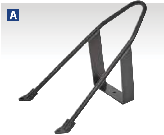
A 170mm Motorcycle Wheel Chock Model No. WCT02 Black powder coated heavy-duty tubular frame. Pre-drilled holes allow chock to be either bolted to floor or trailer to prevent movement and maintain balance. Suitable for motorcycles with up to 170mm wide tyres. Minimum/Maximum Tyre Width: 50/170mm
