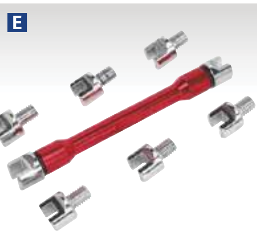
E 9pc Spoke Wrench Set Model No. MS086 Specially designed spoke wrench with eight interchangeable sized heads. Suitable for adjusting spoke tension and correcting buckled wheels. Sizes: 5.4, 5.6, 5.8, 6, 6.2, 6.4, 6.6, 6.8mm
