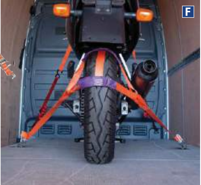
F Motorcycle Rear Wheel Tie Down Model No. TDMCRW Manufactured from polyester webbing. Stitched reinforcement at joins and loops. Suitable for workshop use or for securing motorcycle to flat-bed or trailer. Secures rear wheel to anchor point without compressing the suspension units, thus reducing the risk of seal damage. Ratchet mechanically tensions the webbing using a simple drum and ratchet mechanism for superior load restraint. Load Test: 1000kg Maximum Tension: 500kg Webbing Width: 35mm
