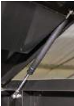
Heavy-duty gas struts on Topchest lid for easy opening.
