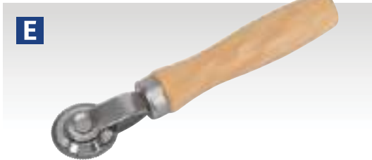
E Patch Stitch Roller Model No. TST15 Designed to roll down inner tube and tyre repair patches to remove trapped air and ensure good adhesion. Features a strong wooden handle. Roller Diameter/Thickness: Ø37/2.5mm
