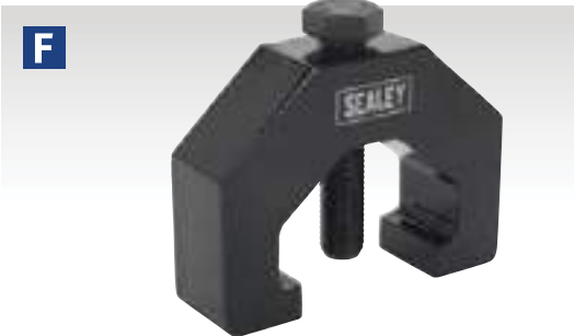
F Steering Drop Arm Puller Land Rover Defender 90, 110, 130 Model No. PS970 Designed to detach the steering drop arm from steering box found on Land Rovers. Size/Spread: 75mm Reach: 23mm
