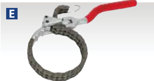
E Ø60-105mm Oil Filter Chain Wrench Model No. VS936 Steel chain wrench with 180° pivoting handle suitable for filters with limited access. Heavy-duty chain with spring locking mechanism for added security. Capacity: Ø60-105mm
