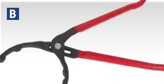
B Ø95-178mm Oil Filter Pliers - Commercial Model No. CV6412 Large forged pliers with chemically blackened finish. Serrated jaws and long handles for extra grip on oily filters. Features a ratchet joint adjustable head. Essential tool for removing commercial filters. Capacity: Ø95-178mm Length: 520mm
