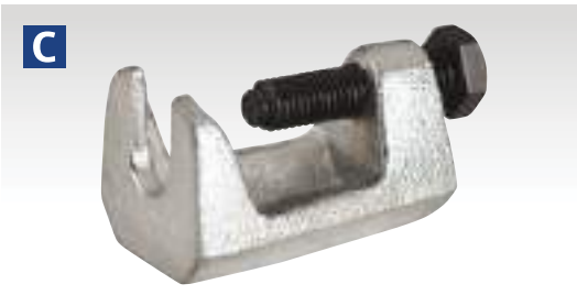
C Ball Joint Splitter Model No. AK380 Forged steel body with steel thrust bolt. Suitable for most small cars and light vans. Jaw Width: 17mm
