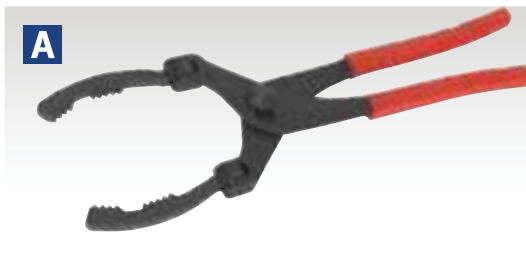
A Ø80-190mm Swivel Jaw Filter Pliers Model No. CV6417 Jaws swivel up to 90° to give access to awkwardly positioned oil, fuel and air brake filters. Chemically blackened finish to prevent corrosion and non-slip grip for added comfort and control. Capacity: Ø80-190mm
