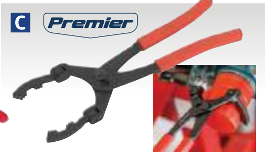
C Ø57-120mm Swivel Jaw Filter Pliers Model No. AK6417 Jaws swivel up to 90° to give access to awkwardly positioned oil and fuel filters. Chemically blackened finish to prevent corrosion and non-slip grip for added comfort and control. Capacity: Ø57-120mm
