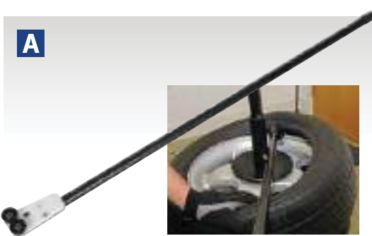
A 1015mm Tyre Bar for Aluminium Wheels Model No. TC963 Tyre bar fitted with nylon ferrules to prevent damage to aluminium wheel rims. Suitable for use with Model No's TC960, TC962, TC965 and other makes of manual tyre changer. Length: 1015mm
