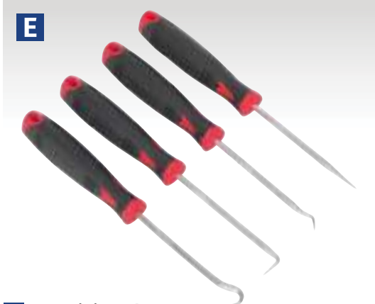
E 4pc Mini Hook & Pick Set Model No. AK5214 Chrome finish shafts with knurling for fingertip precision. Ergonomically styled handles for comfort, grip and accuracy. Suitable for the removal of bushings, cotter pins, O-rings and seals. Contents: Straight, Right Angle, Half-Round, Swan Neck Length: 165mm
