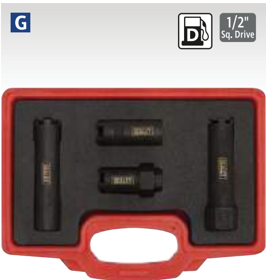
G 4pc Diesel Injector Socket Set Commercial Model No. VS2061 Suitable for the removal and installation of truck and bus diesel injectors. Castellated socket fits common injectors on MAN, Mercedes, Neoplan and Setra. Also suitable for some Iveco, Renault and Scania vehicles. Contents: 1/2"Sq Drive x 72mm x 4-Tooth, 1/2"Sq Drive x 120mm x 3-Tooth, Hex 32mm x 70mm x 4-Tooth (M14 x 1.5mm Receiver Thread), Hex 32mm x 122mm x 4-Tooth for MAN, Mercedes, Neoplan & Setra
