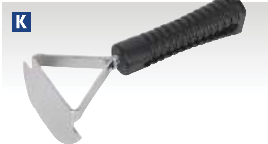
K Tyre Rubber Scraper Model No. TST16 Essential for the preparation of the inside of a tyre. Ensures a clean surface, removing any debris or silicon before buffing. Use with buffing solution.
