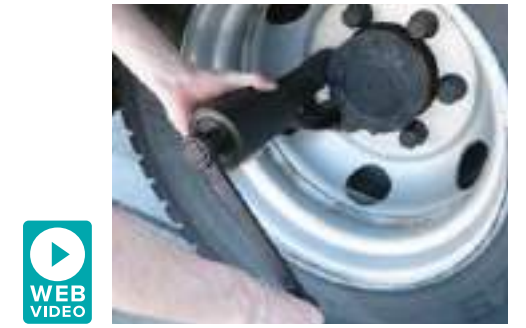
C Torque Multiplier Wheel Nut Wrench 65:1 Model No. SX500 Ideal for removing/installing wheel nuts on commercial and light commercial vehicles when air impact wrench is not easily accessible. Supplied in storage case with two impact sockets and 210mm extension. Output Drive: 1"Sq (Male) Ratio: 65:1 Maximum Rated Output: 6200Nm
