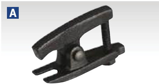
A Ball Joint Splitter Model No. AK381 Chemically blackened forged steel body with thrust bolt. Suitable for most small cars and light vans. Jaw Width: 19mm
