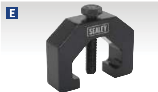
E Steering Drop Arm Puller Land Rover 2, 2A, 3 Model No. PS969 Designed to detach the steering drop arm from the steering box found on Land Rovers. Size/Spread: 60.5mm Reach: 19mm
