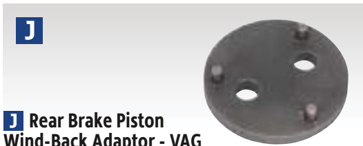
J Rear Brake Piston Wind-Back Adaptor - VAG Model No. VS02821 Adaptor enables retraction of the piston on rear brake calipers when used in conjunction with a traditional wind-back tool with a 2-pin adaptor mounting. 3-pin design suitable for VAG vehicles. Pin Size: Ø3mm Mounting Pin Size: Ø6mm Distance Between Mounting Pin Centres: 20mm Applications: VS0211, VS0240, VS0243, VS028, VS0282, VS0285, VS0286, VS0287
