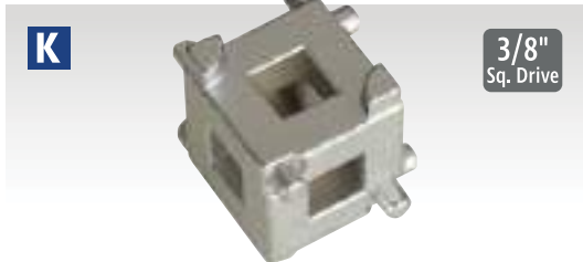
K Brake Piston Cube Model No. VS039 Five possible pin configurations fit US and European applications. Use with 3/8\"Sq drive ratchet wrench and extension bar. Warning: Not for use with impact type ratchets.
