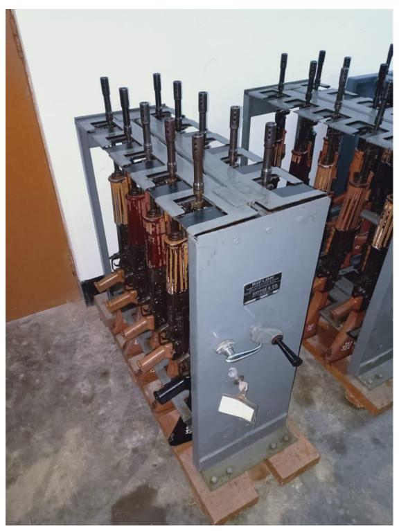
3) **RIFLOK** – **Thief Proof Rifle Racks**, Single Tier type, to accommodate 10 nos of 5.56 INSAS/ 7.62 SLR/AK-47 (Fixed & Side Folding Butt) & 9mm Carbine Rifles **Without ammunition box**.
