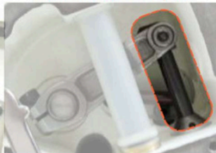
Direct Drive Needle bar system
