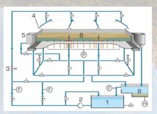
1 storage tank, 2 pump, 3 solenoid valve with timer, 4 nozzle, 5 chamber, 6 experiment tank, 7 chamber, 8 measuring tank; m mass, F flow rate, P pressure
