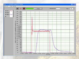
Software Screenshot: water drain for persistent rain with saturation of the soil: red precipitation, blue drain
