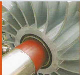
Motor Shaft Coated with Aluma-Coat BR
