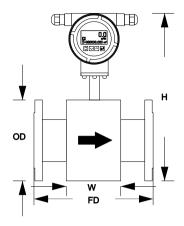
The induced voltage is not affected by the physical properties of liquids like temperature, viscosity, pressure, density and conductivity as long as the conductivity of the measured liquid is above the minimum threshold level. For reliable measurement, the pipe must be completely full of the liquid. The electromagnetic field coil assembly is excited by pulsed DC technique which eliminates the interfering noise and provides automatic zero correction.
