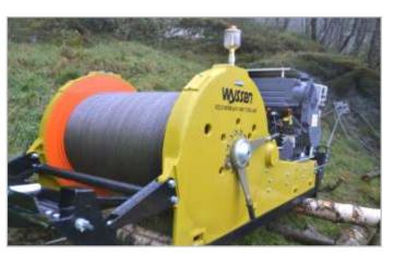
**Cable Winches** are used for driving Cableways as a traction and braking machine to transport Sky-line Crane carriage or the Cableway carriage.
