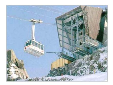
An aerial tramway (Cable Car) is a type of ropeway which uses one or two stationary ropes for support while a third moving rope provides propulsion. With this form of lift, the grip of an aerial tramway is fixed onto the propulsion rope and cannot be decoupled from it during operations.
