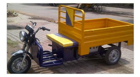
E Rickshaws are three wheel battery operated vehicles, which are considered as an upgrade to conventional rickshaws and are economically better than other fuel variants. These rickshaws, since are battery powered, have zero emission.
