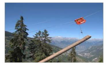
*Carriages* are moved on the main cable with the help of a traction cable on the Cable Winch. The load to be transported is principally attached to the carriage and transported along the cable line.
