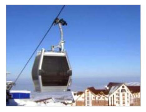
A Gondola lift is a type of ropeway, which is supported and propelled by a single, carrying cum hauling rope. It consists of a loop of a steel cable which is strung between two stations and supported by intermediate towers. The grips of this system could either be fixed or detachable.
