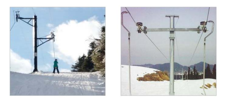
A surface lift is a type of cable transportation system used to transport skiers and snow boarders where riders remain on ground as they are pulled uphill through J-Bars or T-Bars.
