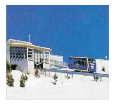
A ropeway, carriers of which are rail borne and rails having the function to support carriers, which are hauled by a haul rope. The track bed could either be sloping or horizontal. The single carrier or in the case of two carriers, both carriers travel forward and backward between the two terminal stations.
