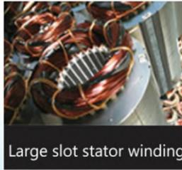
Large slot stator winding
