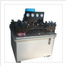
Hydraulic Power Pack
