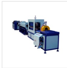
PVC Pipe Plant
