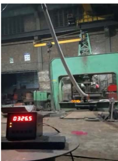
Top load testing of pole
