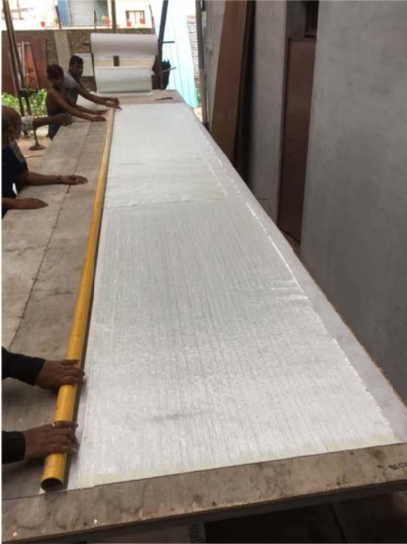
Pole production glass fabric matt winding
