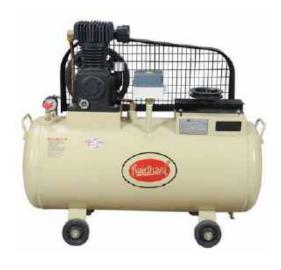
Capacity 36 Liters **Power Supply** Single Phase Maximum Working Pressure : 4kg / cm2 Hydraulic Test Pressure 7kg / cm2 Disc thickness 3 mm Shell Thickness 3 mm HP - 0.5Motor KW 0.37 **AMP**
