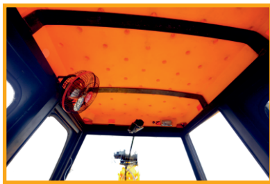
CABIN: Extra protection with heavy bar of cabin roof.
