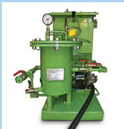
Modified ELC Unit with pre filter, increases efficiency, reduces filtration time, also acts as a coalescer.
