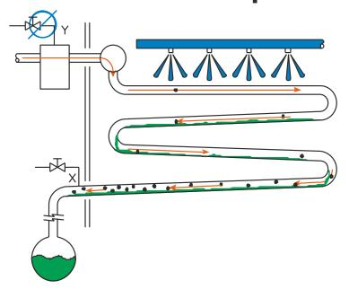
Fig. 1.(left) High velocity of entering refrigerant gas prevents any significant air accumulation upstream from point X. High velocity past point X is impossible because receiver pressure is substantially the same as pressure at point X. Purge from point X. Do not try to purge from point Y at the top of the oil separator because no air can accumulate here when the compressor is running.
