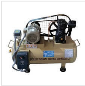
Single Stage Air Compressor
