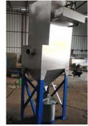
SS Dust Collector System
