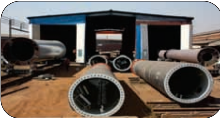
Towers in finished condition coming out of 32 MT Paint Booth
