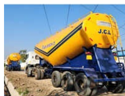
45 Cubic Meter Cement Bulker Trailer
