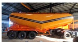
Cement Bulker Truck
