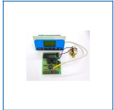
SINGLE COMPRESSOR PID CHILLER
