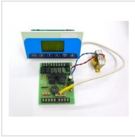
Single Compressor PID Chiller
