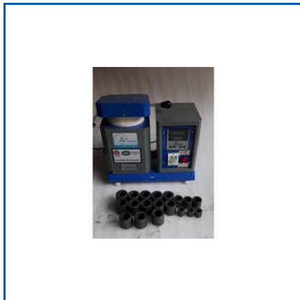
GRAPHITE MELTING FURNACE
