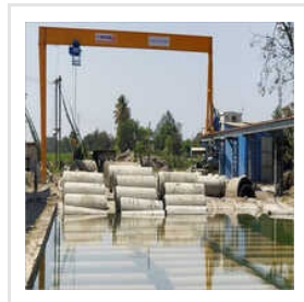
Electric Gantry Crane
