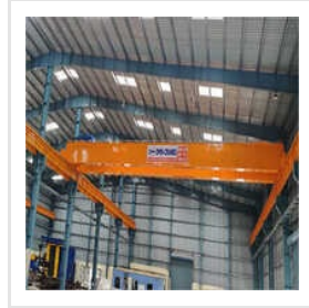
Double Girder Eot Crane
