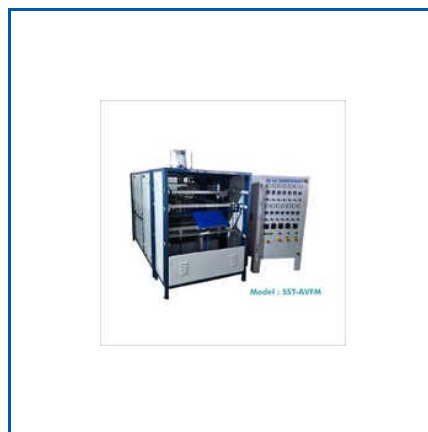
LARGE VACUUM FORMING MACHINE
