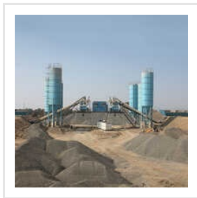
Twin Batching Plant
