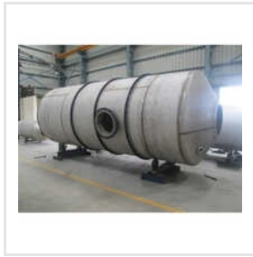
3000 Ltr Mild Steel Storage Tank
