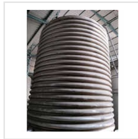
Stainless Steel Chemical Reactor
