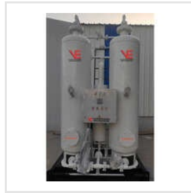
Oxygen Generation Plant
