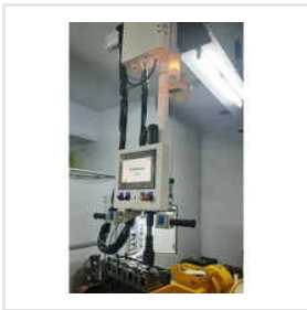
DC Tool Torque Tube Bolt Tightening
