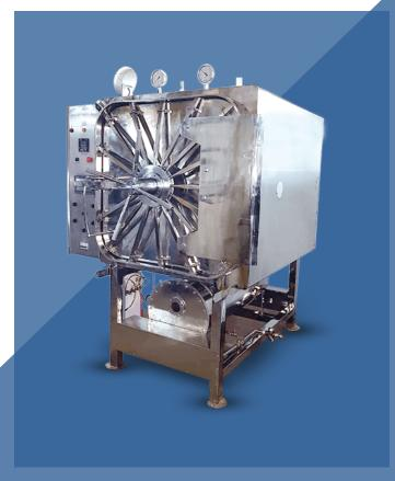
The inner chamber is made of a thick plate of mild steel of non-magnatic stainless steel of 304/316 quality, and the jacket is made from rolled steel. All the sterlizers are hydraulically tested to withstand 2.5 times the working pressure. Fitted with water gauge glass for water level, safty valve, water inlet, and the drain valves. All units are hydraulically tested up to 40 psi. Unit is also fitted with low-water level Cut-off device and automatic pressure cantrol device.
