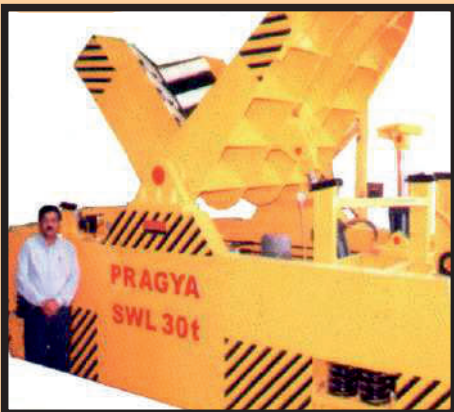
Coil Tilter Cum Trolley up to 70 tons
