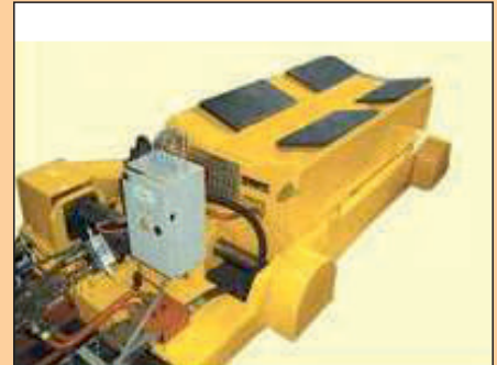
SCISSOR TYPE COIL CAR (HYDRAULIC)
