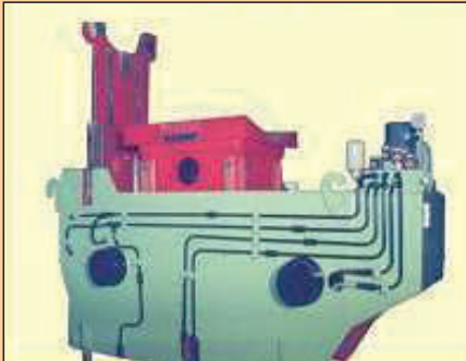
BOX TYPE COIL CAR (HYDRAULIC)
