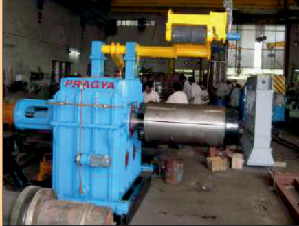
UN-COILER WITH HYDRAULIC EXPAND S COLLAPSE
