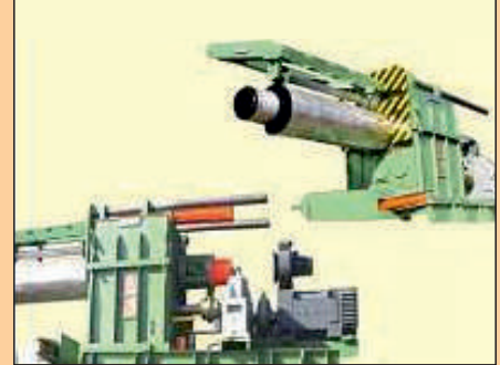
HYDRAULIC RE-COILER UNIT (Capacity 25 MT)
